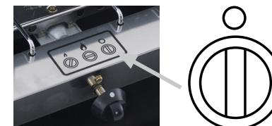
Ensure that all control knobs are in the off position.
